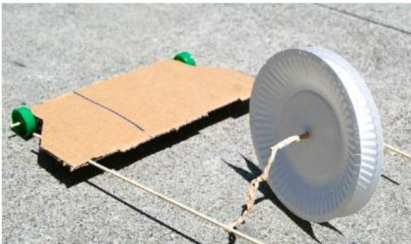
This is another design that uses two paper plates taped back to back instead of CDs for the wheels.
