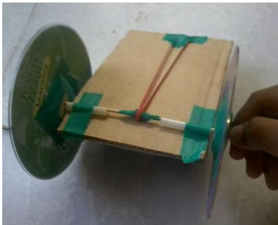
In this design, straws were cut up and taped on top of the cardboard body. The skewer can then slide through the straws instead of through the cardboard. Also, pieces of cardboard are taped over the holes of the CD for the skewers to poke through.
