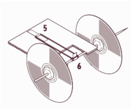
In this design, the skewer is put through the cardboard instead of on top. They used a piece of tape on the skewer to act as a “catch” for the rubber band and also cut a notch in the cardboard body so the skewer could spin freely.
